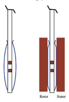
As the rotor stator gap varies, the sensor will detect a change in the distance between the two springs and vary the output on the digital display to indicate the rotor-stator gap.
