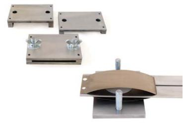
The GMS-750RS is calibrated at the factory prior to shipment. Field calibration is possible. The only requirement is to be able to accurately mimic a 0.250" (6.35mm), 0.500" (12.7mm) and 1.000" (25.4mm) rotor-stator gap. This can be accomplished with a granite surface block, appropriate precision ground spacers, a flat metal plate and the ability to compress the target springs with the flat metal plate (some force is required).
