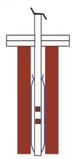
Simply position the stops into the holes provided to limit the maximum depth of the sensor and target springs.
